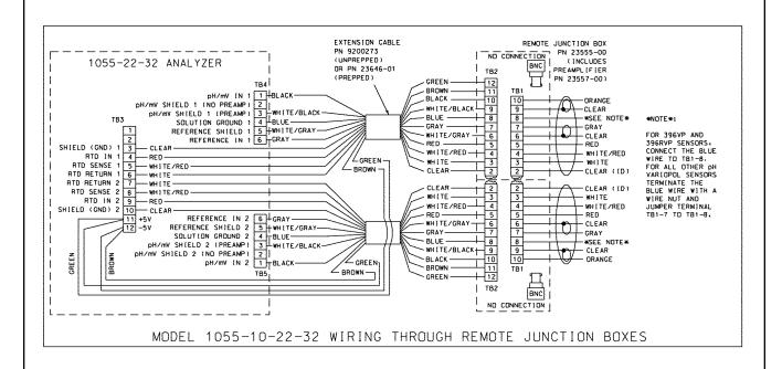
FIGURE 2-36. Wiring Model 396VP-54 to Model 1055-22-32
